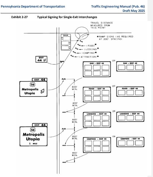
Note: A maximum of four logo sign installations (with a maximum of five specific service types) are permitted at a given interchange approach. In the above figure, an attraction logo may be substituted for any of the other services, provided the appropriate sequencing of signs is maintained. Each panel may be designed to accommodate two, three, four or six logos.
