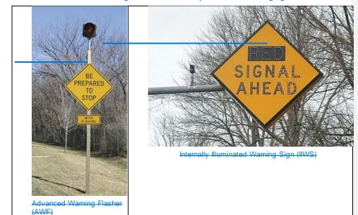
AWF or HWS should only be installed in response to a specifically correctable problem, not in anticipation of a future problem. Generally, AWF or HWS implementation is appropriate only at high speed locations. Before an AWF or HWS is installed, other remedial action should be considered.
